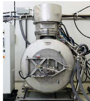
Vacuum Microwave Drying Process
